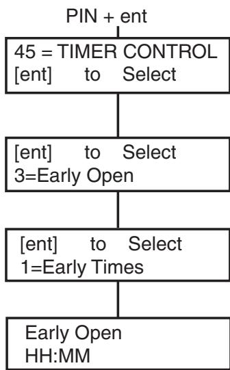
If the **Early Open** option (45.3.2) is enabled, the **Lockout OFF** time for the following day is brought forward by the number of minutes (0 – 240) programmed by the engineer. This allows the system to be manually unset earlier than normal. There are 2 functions within this option:
