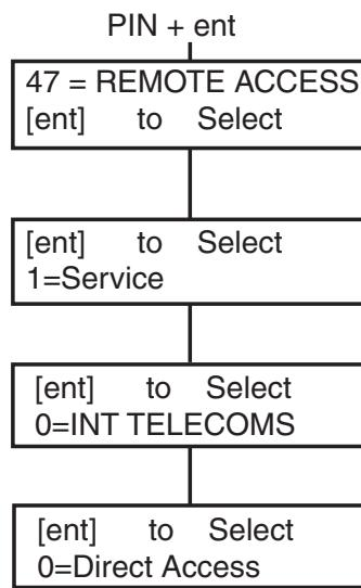
The **1=Service** option enables the user to control the access mode of the remote servicing package. There are 4 communication devices available.
